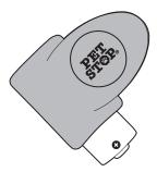
Insert the second 3.6v lithium ion battery in the remote receiver with the (+) terminal facing towards the battery compartment opening. Using a small coin, replace the battery cap turning clockwise.
